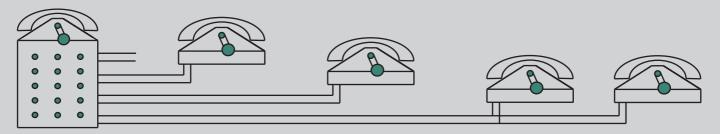
Up to fifteen lines, each connected to one or more magneto telephones, can be branched radially around a manual exchange or annunciator to form a more elaborate network.
